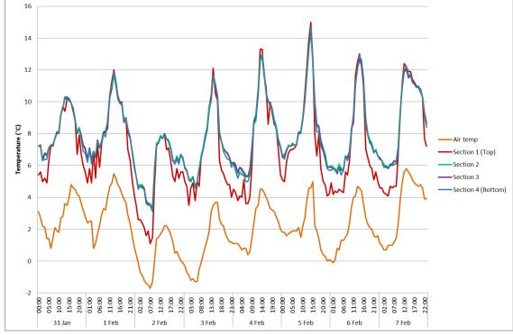
Figure 42: Air temperature and minimum cliff surface temperature by section between 31/01/2015 – 07/02/2015.
