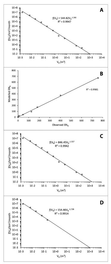
Figure 58: Power law estimation parameters for August to September 2016 (A) frequency density and magnitude of failures for the entire study area, (B) the predicted vs. observed frequency of failures for all binned data, (C) frequency density and magnitude of failures for the unprotected section and (D) frequency density and magnitude of failures for the naturally protected section (shingle beach) [black lines depict best fit models].
