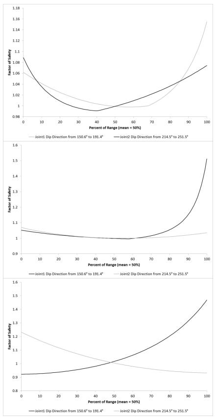
Figure 76: Sensitivity analysis of modelled wedge failures along the defended cliff line in Brighton showing the impact of the range of dip direction for JS1 and JS2 for (A) the 25<sup>th</sup> percentile, (B) the 50<sup>th</sup> percentile and (C) the 75<sup>th</sup> percentile [Note differing scales on y axis].
