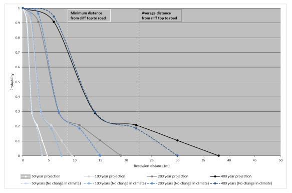
Figure 80: Probabilistic recession model sensitivity analysis accounting for change in future climatic conditions projected for 50, 100, 200 and 400 years for the defended cliff line between Brighton Marina and Saltdean (Minimum and average distance from cliff edge to road identified).
