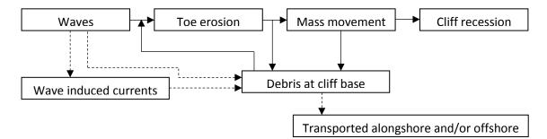
Figure 7: Coastal cliff recession system (Sunamura, 1992, p. 76).
