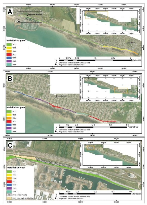
Figure 35: Location and dates for installation of sea defences and cliff stabilisation measures (A) Brighton Marina to Saltdean, (B) Telscombe to east of Peacehaven and (C) detail of Brighton Marina defences.
