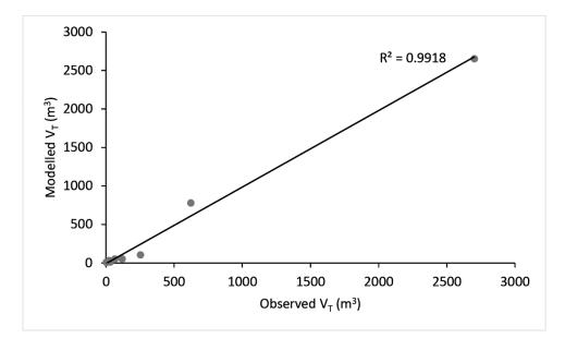
Figure 62: Modelled  $V_T$  vs observed  $V_T$  for the undefended (no beach) section of Telscombe cliffs.
