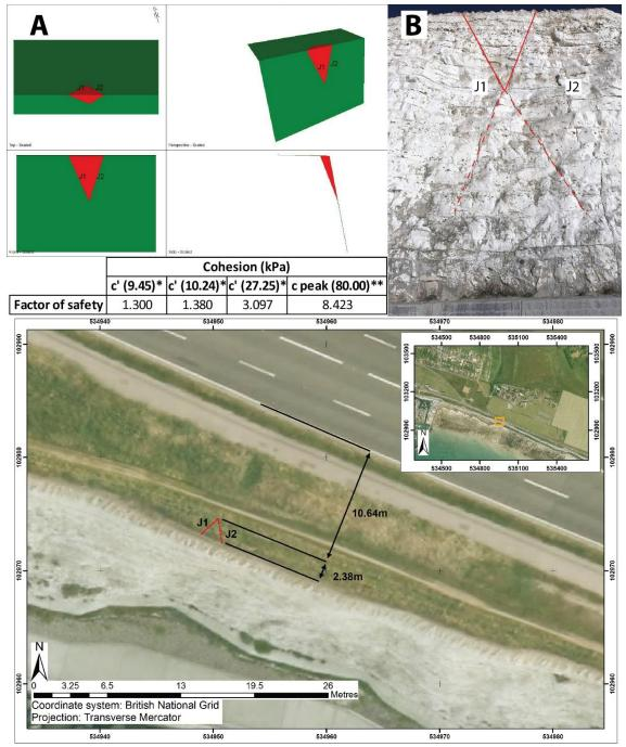
Figure 73: Wedge failure modelling near Roedean School representing the second closest distance from cliff edge to A259 (A) limit-equilibrium modelling in Swedge, (B) field observation with conjugate set identified and (C) cliff top retreat and distance to road (2013 imagery in 'C' downloaded from the CCO) ) [\*cohesion derived from back analysis \*\*cohesion from Barton (1974)].
