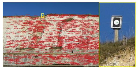
Figure 23: Exterior orientation processing from ADAM 3DM CalibCam Manager view - digitised GCPs (Green) and ROPs (Red) of terrestrial photogrammetry in Brighton Marina on 20.01.2017, inset shows fixed target at cliff top residual scale at x100 for viewing purposes.
