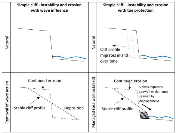
Figure 6: Cliff instability and erosion following the removal of wave action or construction of coastal defences (Adapted from Moore & Davis, 2015).
