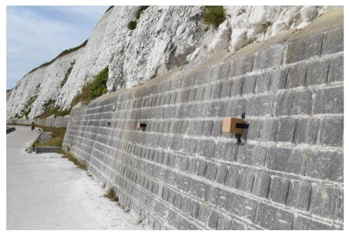
Figure 26: Boxes installed on rear splash wall to determine threshold of detection for terrestrial photogrammetry, Brighton Marina.
