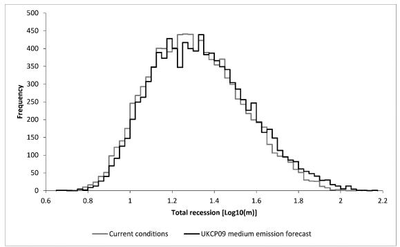
Figure 64: Monte Carlo simulation histogram of Log10 transformation of total recession between 2020 and 2089.
