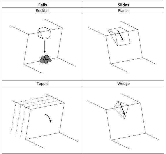
Figure 4: Basic classification of types of rock failure broadly divided into fall and slides (Adapted from Wylie & Mah, 2004).
