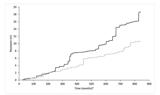
Figure 63: Example of a simulated erosion model for Telscombe run for 840 months (70 years) between 2020 and 2089 (black line indicates future conditions (UKCP09 medium emission scenario, grey line indicates current conditions, \*- time in months from January 2020).
