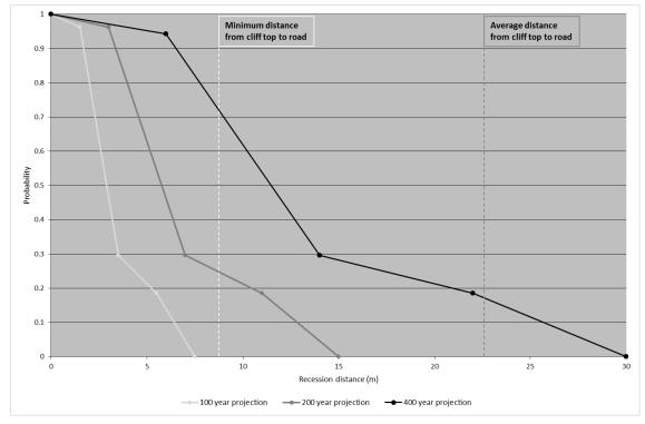
Figure 79: Probabilistic recession model with present climatic conditions projected for 100, 200 and 400 years for the defended cliff line between Brighton Marina and Saltdean (Minimum and average distance from cliff edge to road identified).
