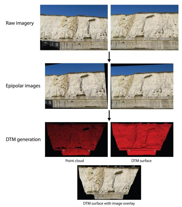
Figure 25: DTM generation workflow from raw imagery to DTM surface with imagery using ADAM 3DM CalibCam and 3DM Analyst (Images taken from Nikon D810 35mm prime lens on 20.01.17
