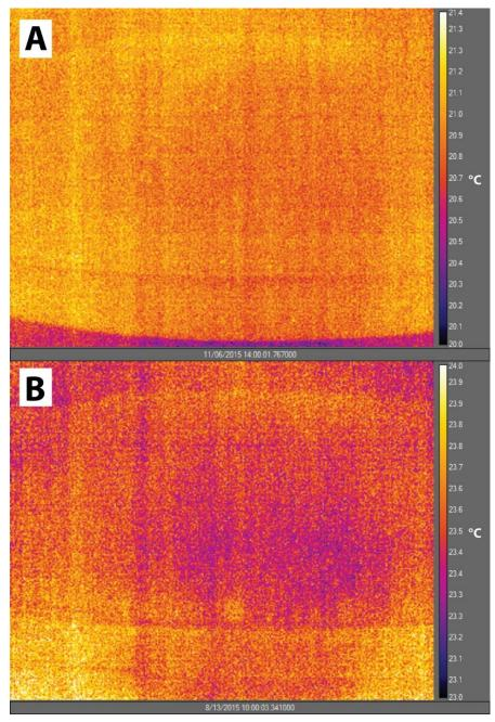
Figure 31: Thermal imagery data capture issues (A) relative humidity exceeding 90% captured on 06/11/2015 at 14:00 and (B) heavy rainfall captured
