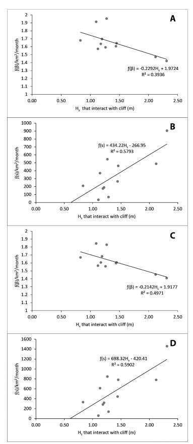
Figure 59: Normalised power law estimation parameters  $\beta$  and s vs. H<sub>s</sub> (A)  $\beta$  vs. H<sub>s</sub> for entire study area, (B) s vs. H<sub>s</sub> for entire study area, (C)  $\beta$  vs. H<sub>s</sub> for the unprotected section of cliff and (D) s vs. H<sub>s</sub> for the unprotected section of cliff (black lines indicate best fit models).
