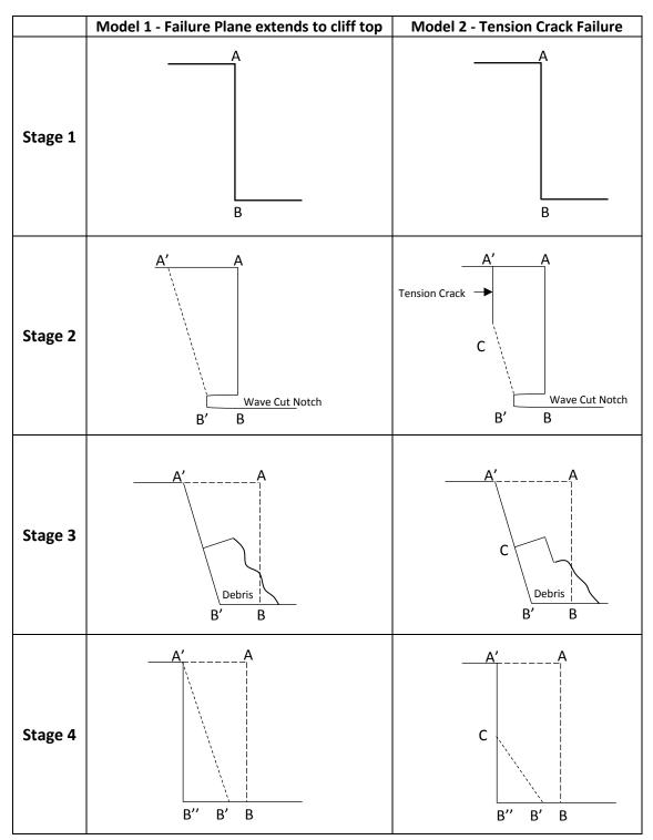
Figure 5: Models for cliff recession due to wave notch development [A- initial position of cliff top, A'cliff top location after failure, B- initial cliff toe position, B'- cliff toe location with debris, B"cliff toe position after debris removed, C- debris extent (Adapted from Sunamura, 1992, p.112).
