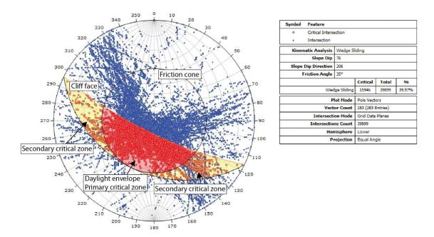
Figure 45: Stereographic representation of discontinuity data for points of intersection between joints and faults for wedge failure.
