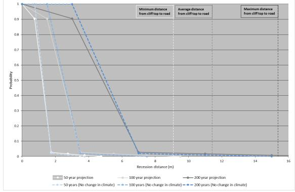
Figure 81: Probabilistic recession model sensitivity analysis accounting for change in future climatic conditions projected for 50, 100, and 200 years for unit 19 (Figure 77) of the defended cliff line between Brighton Marina and Saltdean (Minimum and average and maximum distance from cliff edge to road identified for the unit).
