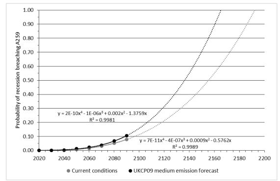
Figure 66: Decadal probability of recession breaching the A259 along the unprotected section of cliff line at Telscombe (dashed lines represent extrapolation beyond model predictions).
