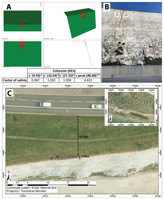
Figure 72: Wedge failure modelling in defended cliffs 700m west of Saltdean (A) limit-equilibrium modelling in Swedge, (B) field observation with conjugate set identified and (C) cliff top retreat and distance to road (2013 imagery in 'C' downloaded from the CCO) ) [\*cohesion derived from back analysis \*\*cohesion from Barton (1974)].
