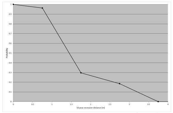
Figure 78: Probabilistic recession model with present climatic conditions projected for 50 years for the defended cliff line between Brighton Marina and Saltdean.
