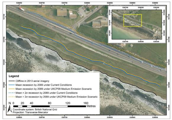
Figure 65: Model predictions of Telscombe cliffline position by 2089.
