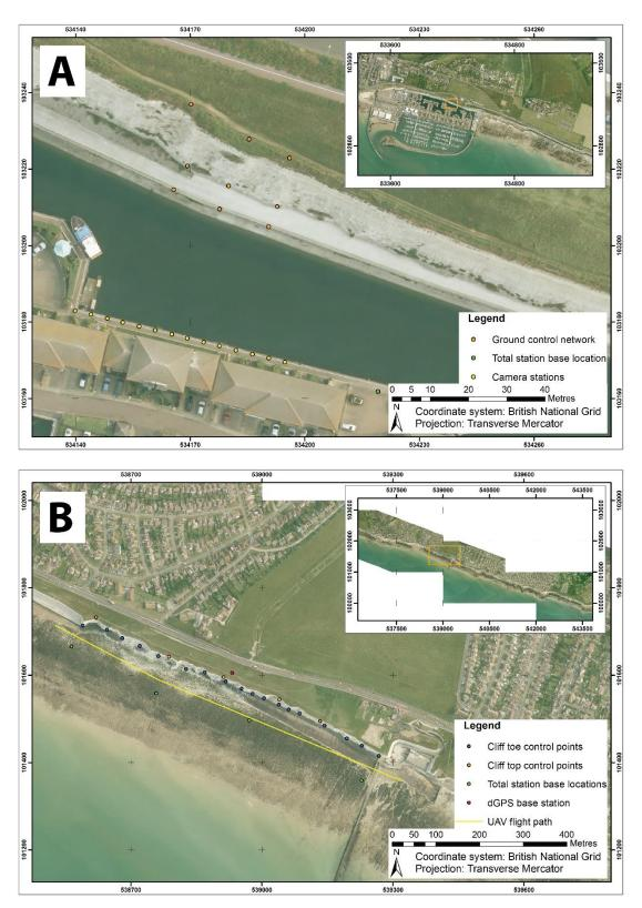
Figure 18: Ground control networks for photogrammetry study sites (A) Brighton Marina and (B) Telscombe (2013 imagery downloaded from the CCO).
