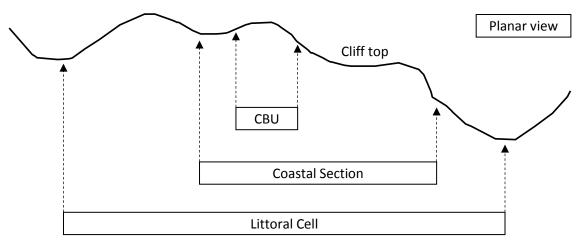
Figure 13: The Cliff Behaviour Unit framework (Adapted from Lee & Clark, 2002, p. 11).
