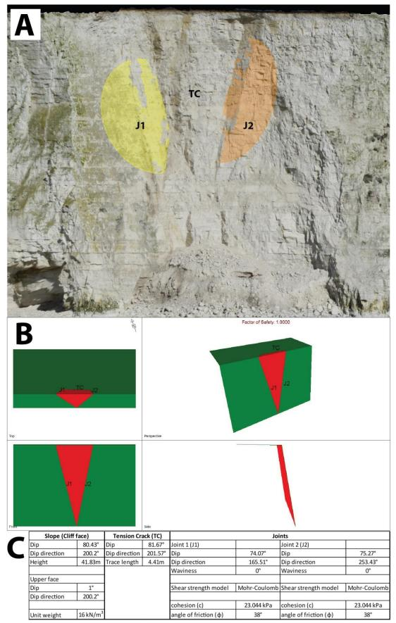
Figure 56: Limit equilibrium model of wedge failure between February and March 2017 using Swedge, (A) 3D model in ADAM 3DM Analyst detailing the joint surfaces, (B) Model output from Swedge, (C) Tabulated input parameters for Swedge analysis.
