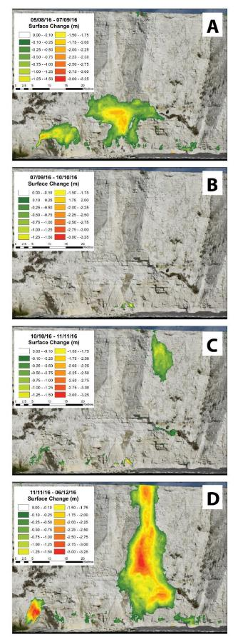
Figure 51: Surface change monitoring successive failures in the Newhaven Chalk at Telscombe between 05/08/16 and 06/12/16, cell size=0.10m (A)Aug-Sep 2016, (B)Sep-Oct 2016, (C) Oct-Nov 2016 & (D) Nov-Dec 2016.
