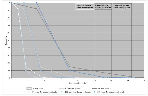
Figure 82: Probabilistic recession model sensitivity analysis accounting for change in future climatic conditions projected for 50, 100, and 200 years for unit 6 (Figure 77) of the defended cliff line between Brighton Marina and Saltdean (Minimum and average and maximum distance from cliff edge to road identified for the unit).
