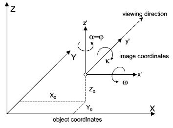
Figure 22: Exterior orientation rotation parameters for terrestrial photogrammetry (Source: Luhman et al., 2011, p. 204 Figure 4.3).
