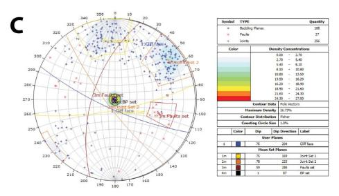
Figure 44: Wolf equal angle stereographic projection of discontinuity data from Telscombe cliffs, (A) pole plot densities of all mapped discontinuities, (B) pole plot densities of mapped joints and faults, and (C) pole plot densities of all mapped discontinuities with identified joint and fault sets with great circles.
