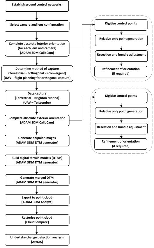
Figure 17: Digital photogrammetry workflow for terrestrial and UAV applications [software platform used].
