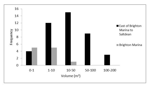
Figure 69: Frequency of different volumes for potential wedge failures generated from observed conjugate joint sets between Brighton Marina and Saltdean.
