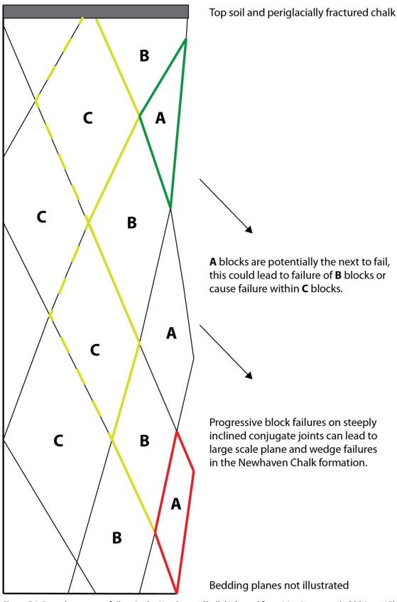
Figure 54: Peacehaven type failure in the Newhaven Chalk (Adapted from Mortimore et al., 2004a, p.15) illustrating the progressive nature of failures observed at Telscombe between August and December 2016 (Red – Aug-Sep, Green – Oct-Nov and Yellow – Nov-Dec).
