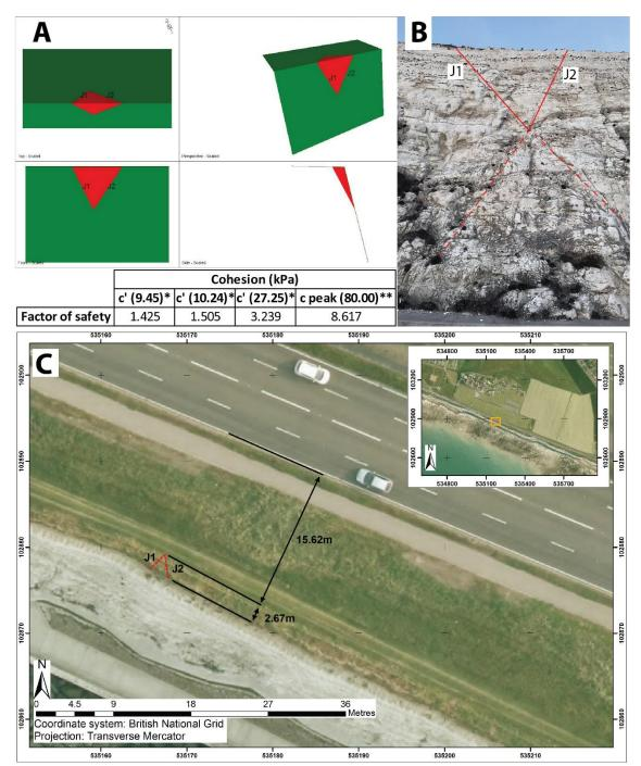
Figure 74: Wedge failure modelling near Roedean School representing the third closest distance from cliff edge to A259 (A) limit-equilibrium modelling in Swedge, (B) field observation with conjugate set identified and (C) cliff top retreat and distance to road (2013 imagery in 'C' downloaded from the CCO) [\*cohesion derived from back analysis \*\*cohesion from Barton (1974)].
