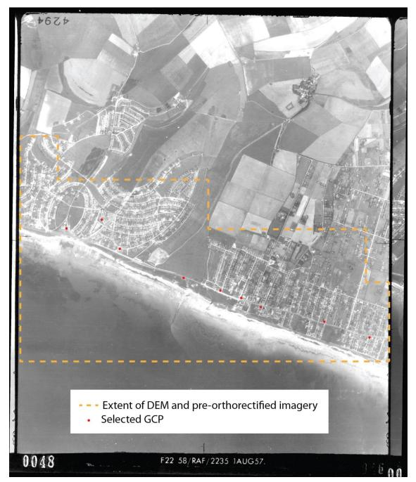
Figure 16: Orthorectification exterior orientation example, Saltdean 1957.
