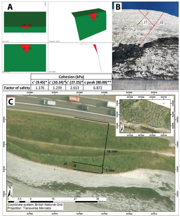
Figure 71: Wedge failure modelling in defended cliffs 500m west of Saltdean (A) limit-equilibrium modelling in Swedge, (B) field observation with conjugate set identified and (C) cliff top retreat and distance to road (2013 imagery in 'C' downloaded from the CCO) ) [\*cohesion derived from back analysis \*\*cohesion from Barton (1974)].
