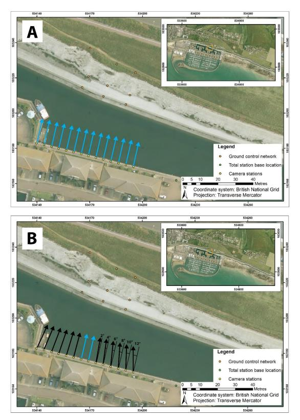
Figure 19: Terrestrial photogrammetry image capture procedures (A) strip and (B) converging image set (2013 imagery downloaded from the CCO).
