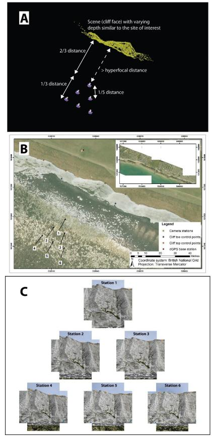
Figure 21: Interior orientation/ calibration set up (A) ADAM 3DM CalibCam 3D view of stations and relatively only points (yellow point cloud) with approximate spacing labelled, (B) Ground control network and camera direction and (C) landscape and portrait images from each station captured from Nikon D810 35mm fixed lens with cliff top targets marked in orange and cliff toe points in blue. (2013 imagery in (B) downloaded from the CCO).
