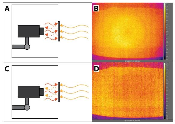
Figure 30: Thermal image flattening undertaken on 18/12/2014 (A) schematic illustrating reflected operating temperature being recorded (B) thermal image illustrating the reflected operating temperature of the camera, (C) schematic illustrating the corrected thermal recording and (D) the corrected thermal imagery (Temperatures on legends in (B) and (D) are in °C).
