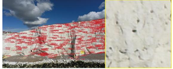
Figure 24: Example of digitised flint in ADAM 3DM CalibCam – point number 26, image captured from UAV flight on 10.10.16 (Red points and numbers are ROPs, green line in insert is residual for point 26 with a visual scaling factor of x100).
