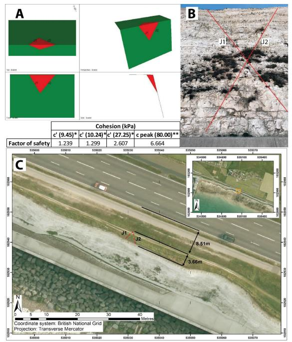
Figure 70: Wedge failure modelling in defended cliffs near Roedean School (A) limit-equilibrium modelling in Swedge, (B) field observation with conjugate set identified and (C) cliff top retreat and distance to road (2013 imagery in 'C' downloaded from the CCO) ) [\*cohesion derived from back analysis \*\*cohesion from Barton (1974)].
