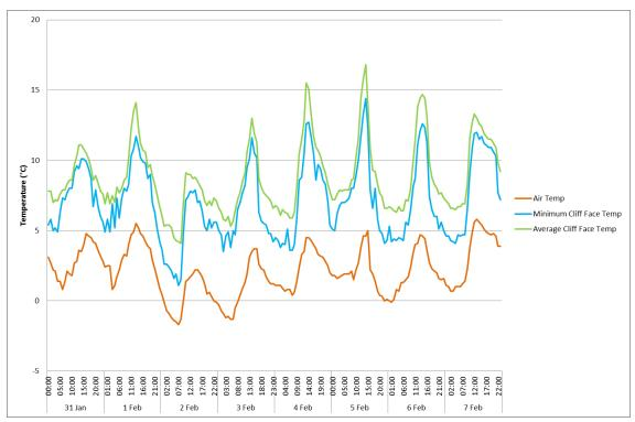
Figure 41: Air temperature, average cliff face temperature and minimum cliff face temperature between 31/01/2015 and 07/02/2015.
