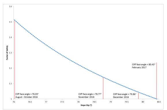
Figure 57: Limit equilibrium analysis of wedge failure in Newhaven Chalk, Telscombe effect of toe erosion in steepening of cliff face on Factor of Safety (FoS) using Swedge between August 2016 and February 2017.
