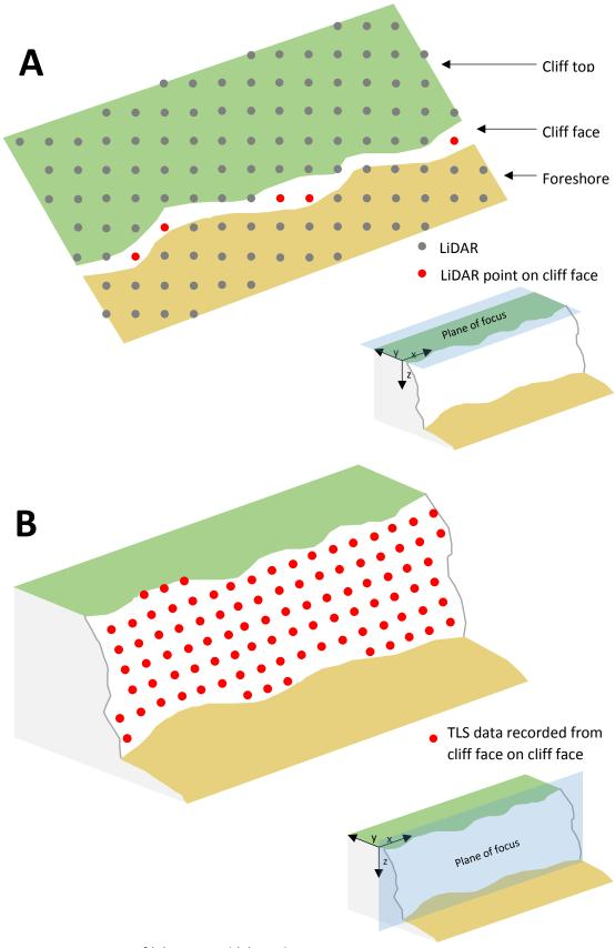
Figure 9: Comparison of (A) LiDAR and (B) TLS data capture.
