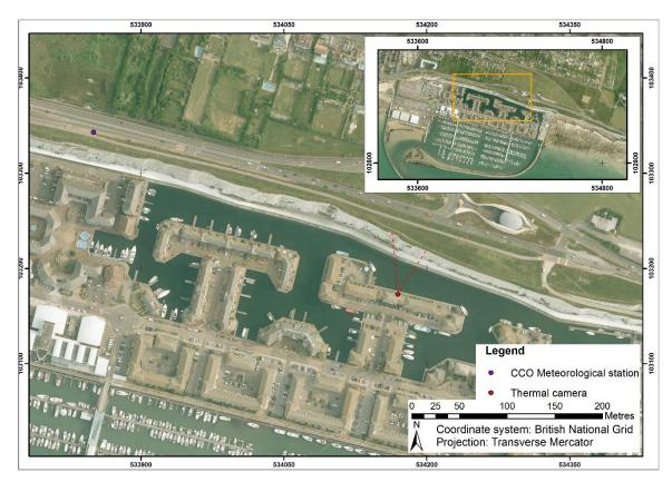
Figure 28: Location of thermal camera and meteorological station at cliffs in Brighton Marina (Red dashed line indicates the approximate field of view of the thermal camera) [2013 imagery downloaded from the CCO].
