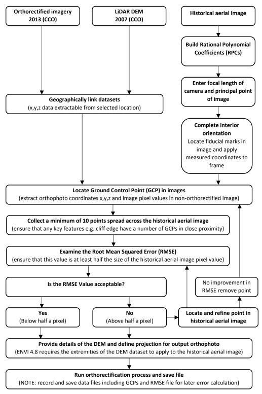
Figure 15: Orthorectification workflow using ENVI 4.8.
