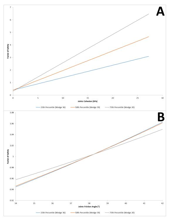
Figure 75: Sensitivity analysis of modelled wedge failures along defended cliff lines in Brighton using the 25th, 50th and 75th percentile of wedges with reference to FoS value, (A) joint cohesion varied from 0-27.25 kPa and (B) joint friction angle varied from 34°-42° [Note differing scales on y axis].
