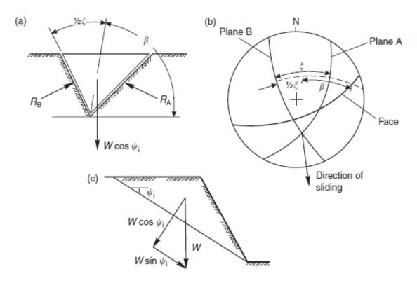
Figure 12: Resolution of forces to calculate factor of safety of wedge: (A) view of wedge looking at the slope face which shows the definition of angles  $\beta$  and  $\xi$ , and reactions on sliding planes R<sub>A</sub> and R<sub>B</sub>, (B) stereonet showing measurement of angles  $\beta$  and  $\xi$ , (C) cross-section of wedge showing resolution of wedge weight W (Source: Wylie & Mah, 2004, p. 156).
