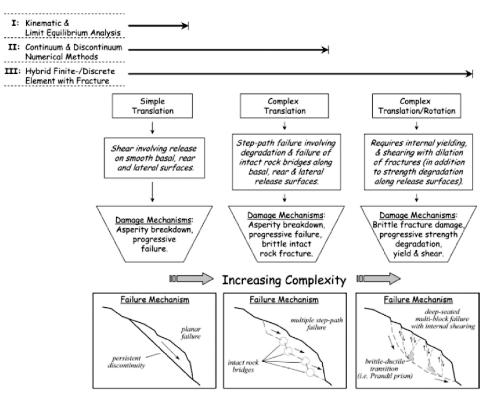
Figure 10: Levels of landslide analysis and mechanisms of failure (Stead & Coggan, 2012, p. 145 after Stead et al., 2006).
