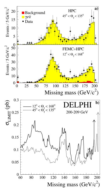
Figure 6: a) The distributions of the missing mass for the events at 200-209 GeV in the HPC and in the FEMC+HPC. The light shaded area is the expected distribution from  $e^+e^- \to \nu\bar{\nu}\gamma$  and the dark shaded area is the total background from other sources. b) Upper limits at 95% C.L. and at 205 GeV (within the quoted solid angles) for the production of a new unknown stable neutral object .
