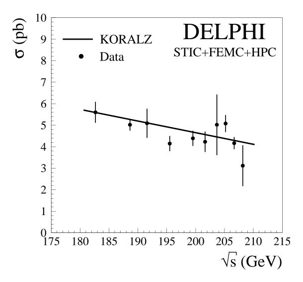
Figure 3: The single-photon cross-section measured by the STIC, FEMC and HPC detectors compared to the cross-section predicted by Koralz.
