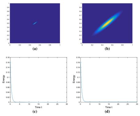
Fig. 3 Computational steady state of the Fokker–Planck model and energy decay for w=1 in the case of no and little diffusion strength. a Steady state (top view)—no diffusion. b Steady state (top view)—with diffusion. c Energy decay in the case of no diffusion. d Energy decay in the case of diffusion
