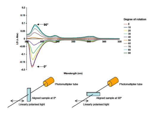
Figure 4.8. LD spectra from an inherently aligned sample of GNNQQNY crystals at 10° interval tilts. The schematic below shows the position of the cuvette at 0° and 90°. See chapter 6 figure 6.6 for further experimental details.
