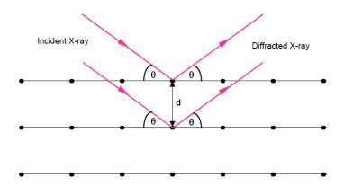
Figure 2.11. Interaction of X-rays with a crystal lattice illustrating Bragg's law.
