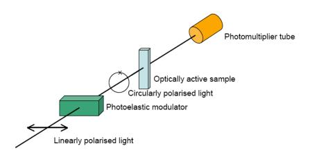
Figure 2.1. Experimental setup inside a CD spectrometer.
