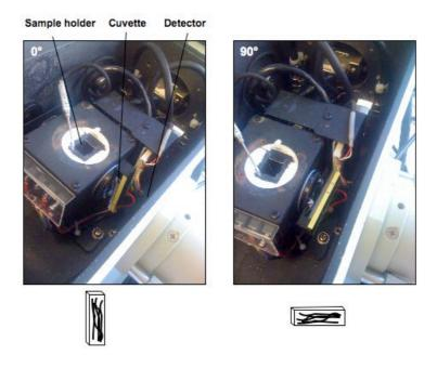
Figure 6.6. Sample set-up for determining degree of alignment of amyloid species within the cuvette and whether linear dichroism is contributing to CD spectra. Previous CD readings were taken with the sample in the cuvette and held in position in the sample holder. Here, readings were taken with the cuvette placed at the end of the sample holder, closer to the detector, where the cuvette could then be rotated 90°.
