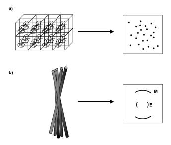
Figure. 2.13. Schematic showing X-ray diffraction of a) crystals and b) a bundle of aligned fibres. M refers to meridional, E refers to equatorial.
