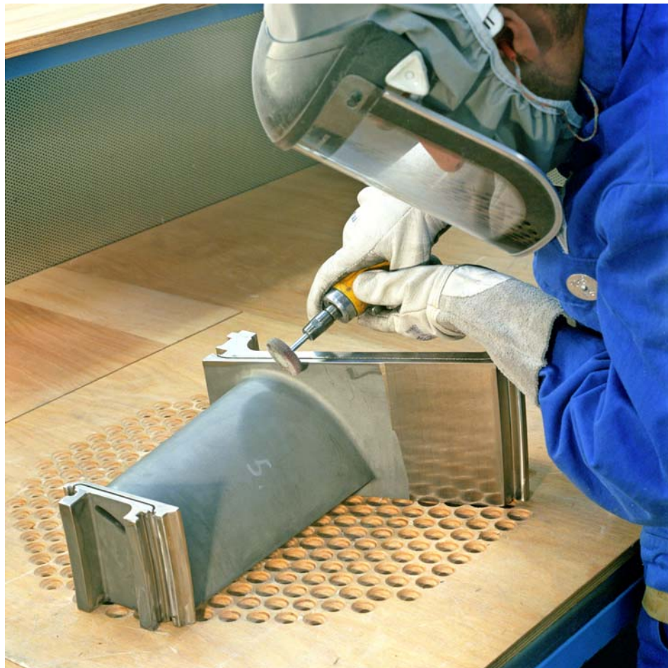
Figure 5.2: Deburring Gas Turbine Blade Edges, Which Can Only Be Performed Manually Courtesy of Siemens Presspicture
