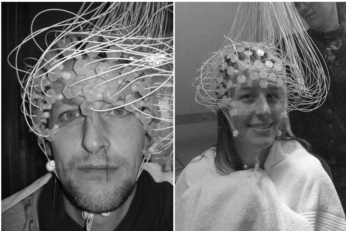
Figure 2-7: 128 channel Geodesic sensor net worn by models.
