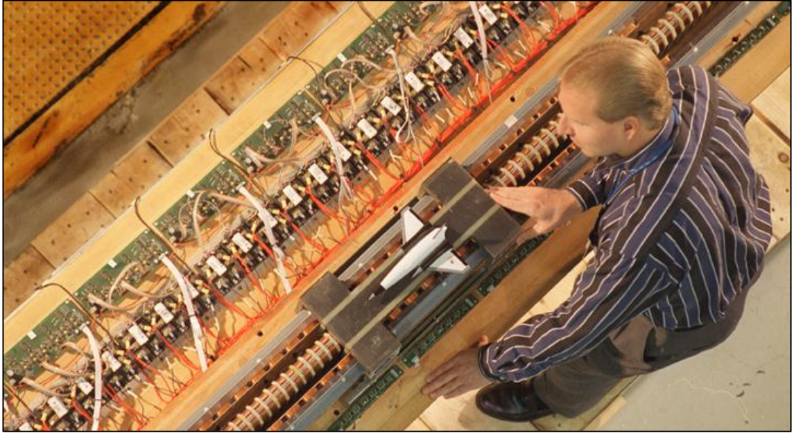
Figure 16: Carrier and vehicle being prepared on Marshall's experimental track
