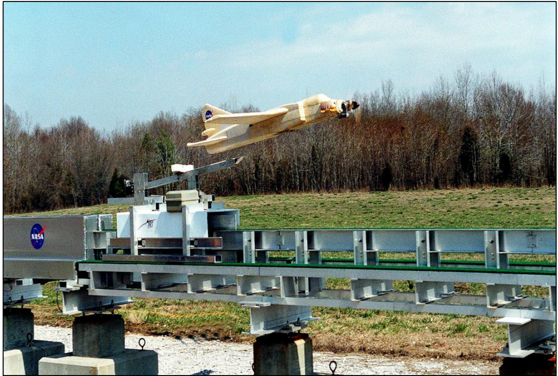
Figure 17: 1/9 subscale vehicle model clearing MLAS demonstration track
