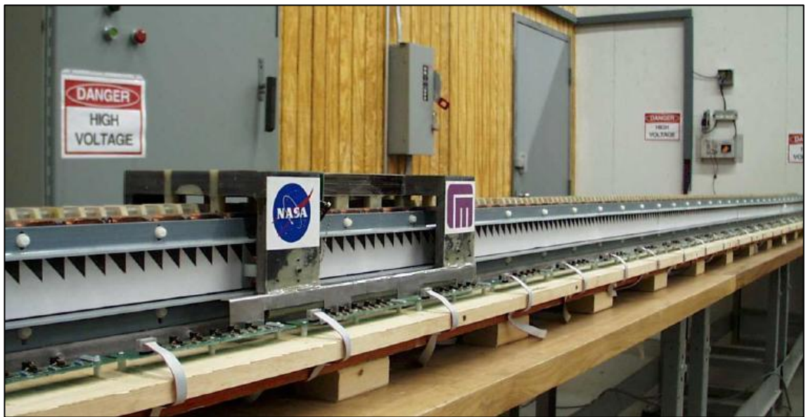
Figure 18: Foster-Miller Inc. test track close up of drive section and test vehicle
