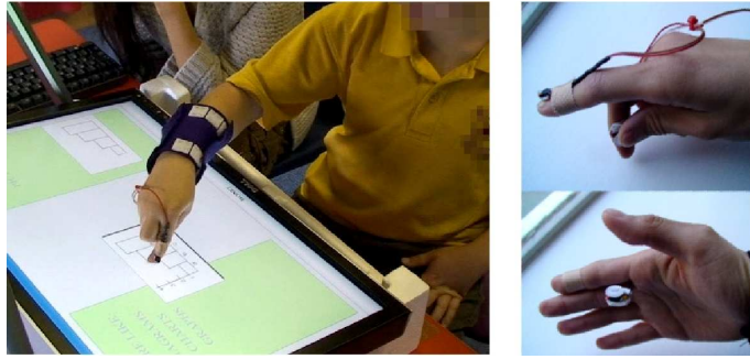
Figure 3.6: Student using the infra-red finger tracking device (left side), a close-up of the infra-red LED on a finger (top-right) and the microswitch (bottom-right).
