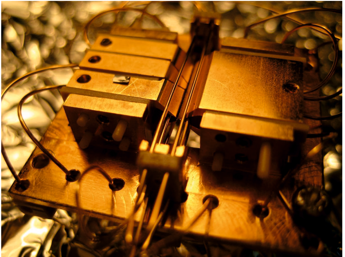
Figure 3.10: Picture of the assembled blade trap with wiring and mounting plate.
