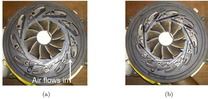
Figure 1.2: Inside of a Garrett GT3782VA 84 Trim *090A/R variable geometry turbocharger. (a) Fully opened vanes, (b) Fully closed vanes.
