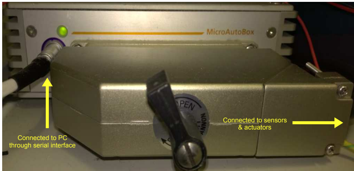
Figure A.3: MicroAutoBox connections to PC, sensors and actuators.
