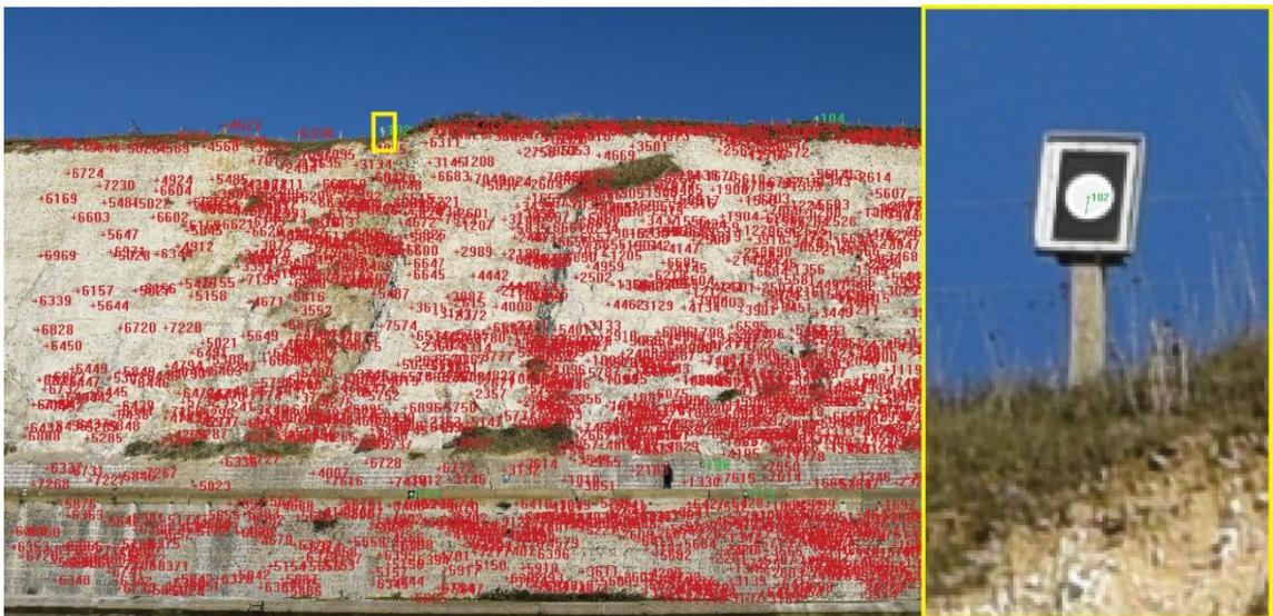
Figure 23: Exterior orientation processing from ADAM 3DM CalibCam Manager view - digitised GCPs (Green) and ROPs (Red) of terrestrial photogrammetry in Brighton Marina on 20.01.2017, inset shows fixed target at cliff top residual scale at x100 for viewing purposes.
