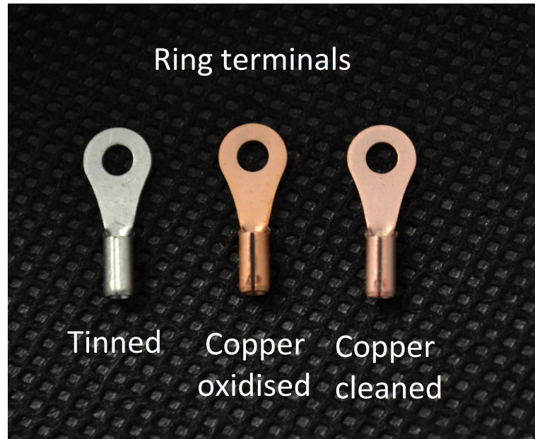
Figure 7.8: Stages of stripping tin from copper
