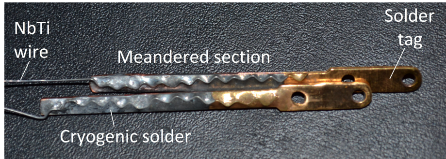
Figure 7.16: Meandered section of NbTi on a solder tag
