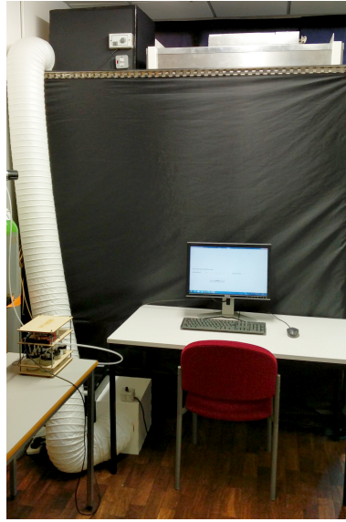
Figure 8.4: Olfactory interaction space: clean room wrapped into a black water repellent fabric with an air extractor E1 and the clean air blower on the top, as well as a scent-delivery device and an air extractor E2 in the bottom-left corner (outside the clean room).
