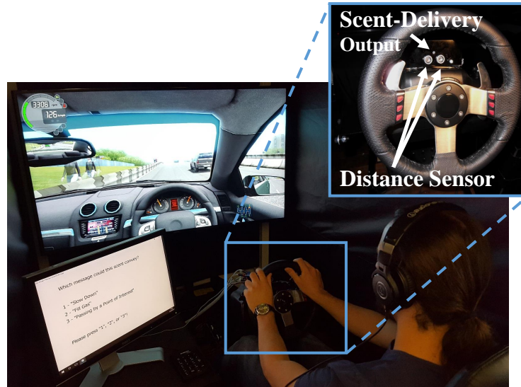
Figure 9.6: Setup of the driving simulator with an integrated system of automated scent-delivery used for the mapping task.
