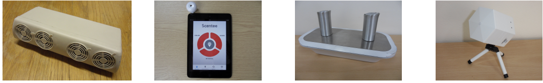
Figure 7.3: Scent-delivery devices (from left to right): Vortex Activ USB, Scentee on an iPad, oPhone DUO, Aroma Shooter.
