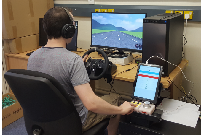
Figure 2.6: The experimental setup of the touchscreen interface used in lab-based study conducted by Ng et al. [146]. Participants had to keep the virtual vehicle in lane as accurately as possible while interacting with the touchscreen.
