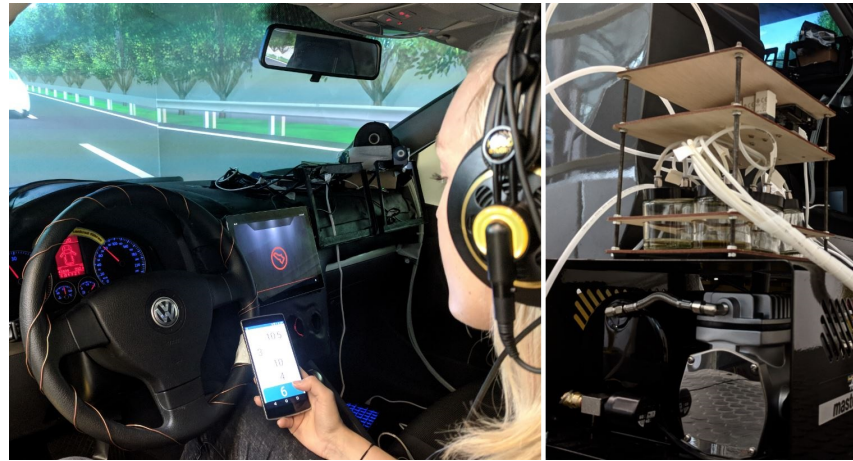
Figure 12.1: Study setup: Participants had to frequently intervene by actuating the brake pedal in case the automated longitudinal system fails (low reliability indicated on the central in-vehicle display), while performing a detection-response task on a smartphone (left). To hide the activation sound of the olfactory device (located outside the vehicle, right), we used noise-cancelling headphones for the sound output of the driving simulation.
