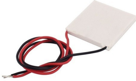
Figure 2.7: A Peltier element. It allows to deliver cold on one side and warm on the other depending on the current direction.
