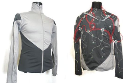
Figure 2.2: A tactile jacket to enhance films. It embeds 64 actuators, allowing complex patterns to be display to users while they watch movies [12].
