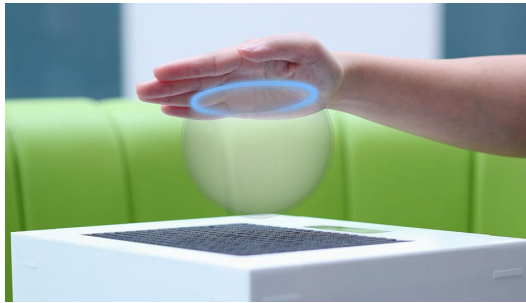
Figure 2.17: Representation of the display of a 3D shape using UMHs [18].
