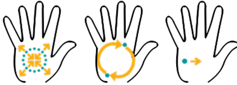
Figure 3.5: Haptic patterns for the Full Stop painting. Main Tate Sensorium pattern (left), and two alternating haptic patterns (middle ‘simple circle’ and right ‘line’). In the Main Tate Sensorium pattern, there is a circle shape composed of 16 points of varying size (having an increase/decrease in diameter of the formed circle), synchronized with the rain pattern.
