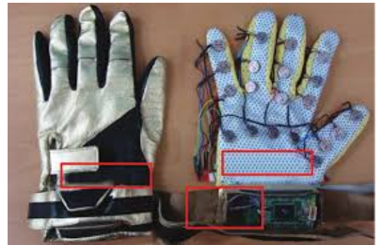
Figure 2.3: Vibrotactile Haptic gloves. It embeds a grid of actuators to mirror the content of a movies [23].
