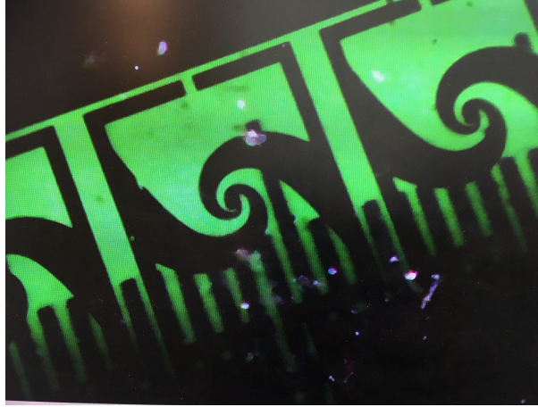
Figure 3.4: Optical image of the spiral antenna with 300 nm thick gold printed on a plastic substrate. The ticks on the scale are 100 \mu\text{m}
