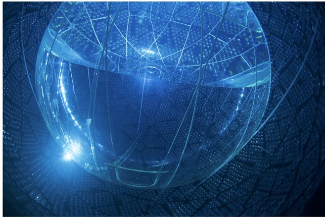
Figure 3.2: A photo of the SNO+ detector during the partial fill. Here the interface between the liquid scintillator and UPW is visible.
