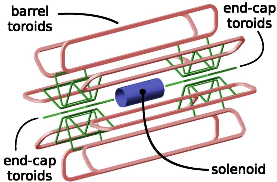
Figure 2.6: Schematic representation of the [ATLAS](#) magnet system. [77]
