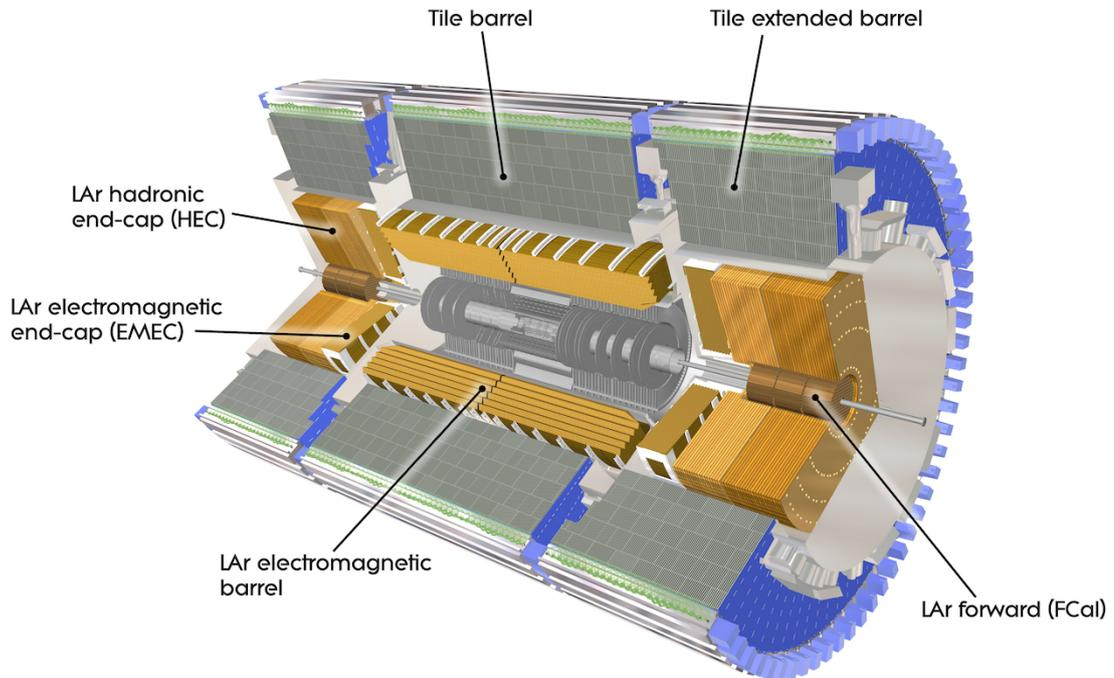
Figure 2.8: Schematic view of the *ATLAS* calorimetry system. [61]
