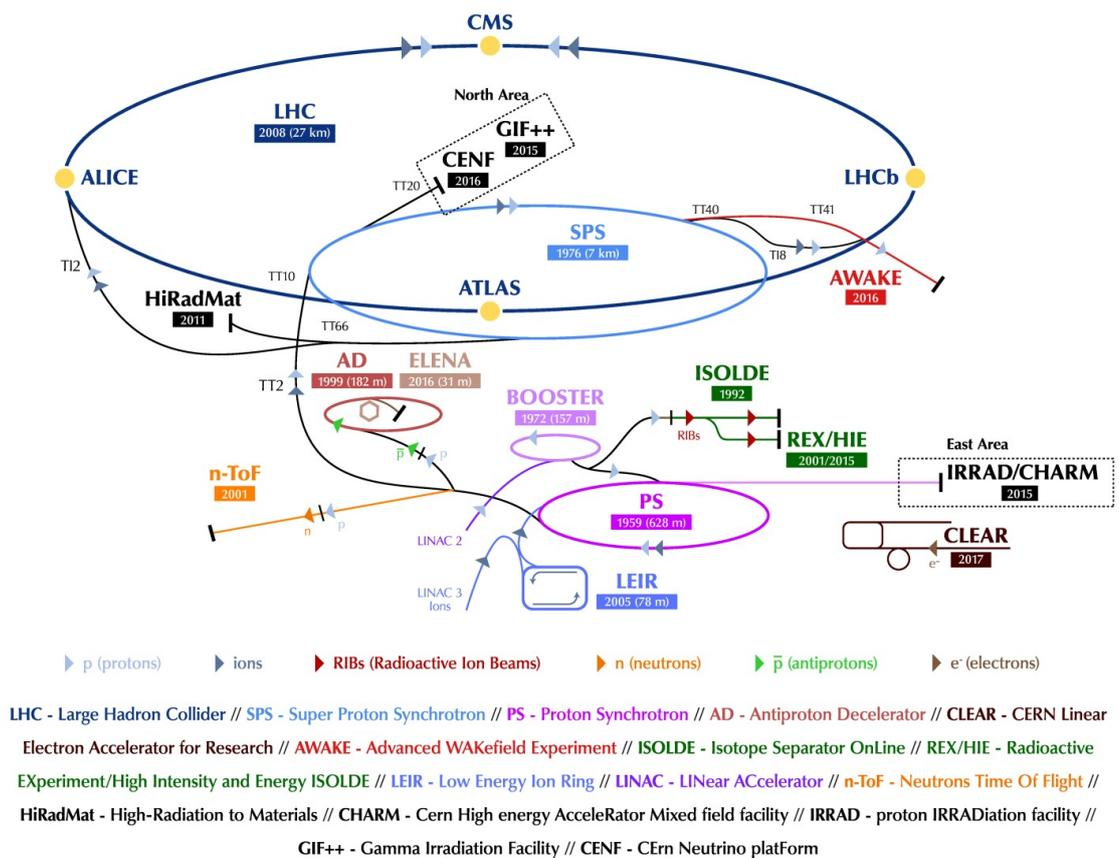
Figure 2.1: Schematic representation of the CERN acceleration complex. [69]
