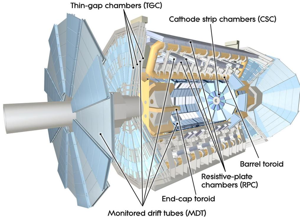
Figure 2.9: Schematic view of the [ATLAS](#) Muon Spectrometer. [61]
