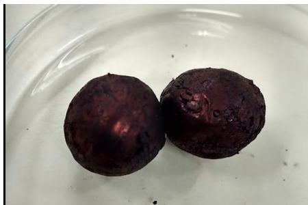
**Figure 4-7** Cy5 **3-8b** reaction with Indole **4-15** after 60 minutes oscillation in the MM400 forms a sticky coating on the ZrO<sub>2</sub> balls.
