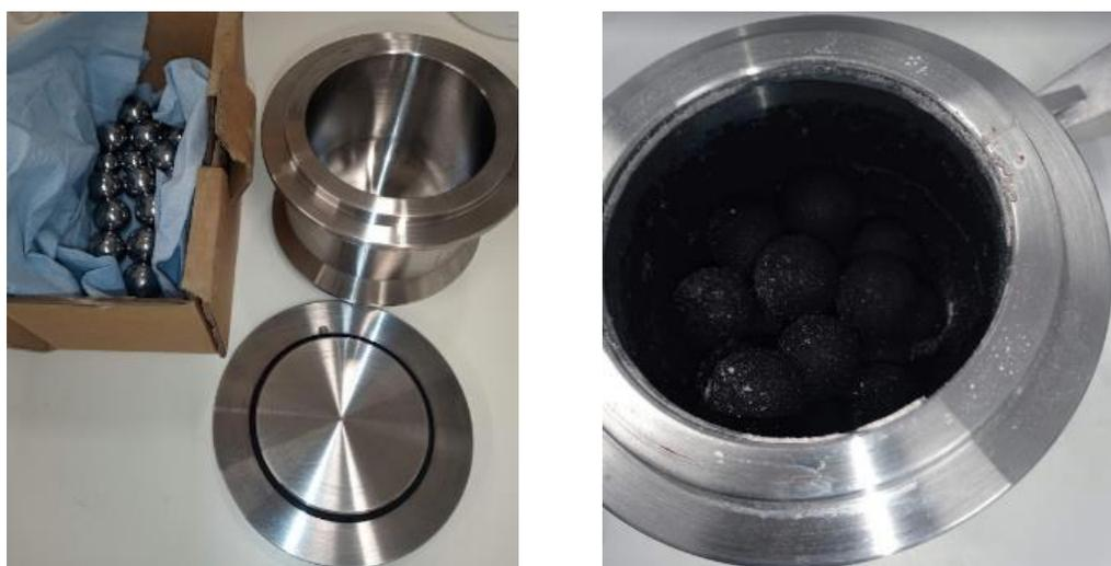
**Figure 4-13** Top: the starting reagents Bromoaniline **3-1g**, sodium acetate, Zincke salt **1-1** – the indole is in the jar at the rear – it is a pale pink crystalline solid. Bottom: (L) The 125 mL Stainless Steel PBM and milling balls and (R) the crude reaction mixture after 60 minutes in the PBM
