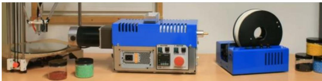
**Figure 5-16** The FilaFab 350 Pro EX, designed to extrude filament ready for 3D printing<sup>232</sup>
