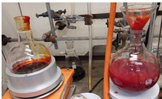
**Figure 3-8** (Left flask) Crude product dissolved in methanol, (Right flask) precipitation into warm diethyl ether
