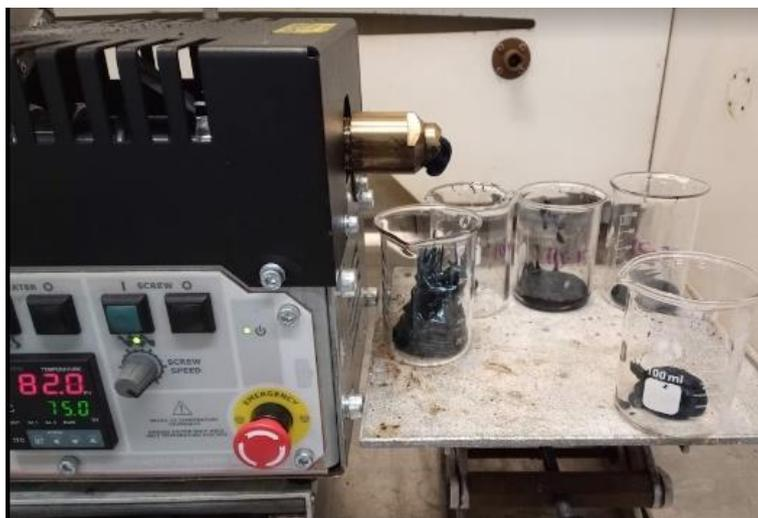
**Figure 5-21** Quality control: collecting separate fractions for analysis
