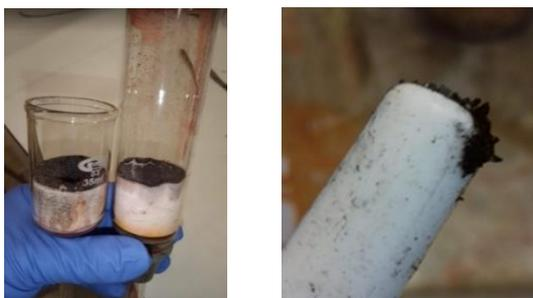
**Figure 3-10** (L) The result of filtering the crude through celite after activation in WC vessels, and (R) the magnetic property of the filtered solid with a magnet retriever
